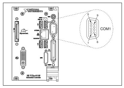
Figure 3-3. COM1 Connector Location and Pinout
